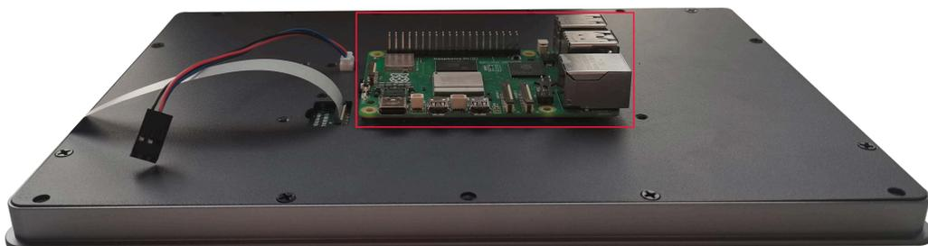
6. Pass the FPC cable through the reserved hole on the heat sink, insert it into the CAM/DISP1
