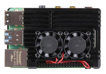
4. Now, turn the Raspberry Pi 4 with the top around, put the bottom part onto it and screw the case tight at the bottom with the screws
